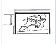
Powered craft, particularly with twin engines, will benefit enormously from 'double decking' insulation, with a 6" gap between layers.
