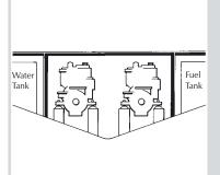
Avoid leaving noise caverns either side of the engine. Drop a removable bulkhead beside the engine and insulate this. Remember, fuel and water tanks collect and amplify noise.
