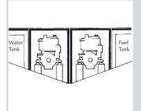
With twin engines in a new vessel, try to put each engine in a separate compartment with a removable bulkhead between.
